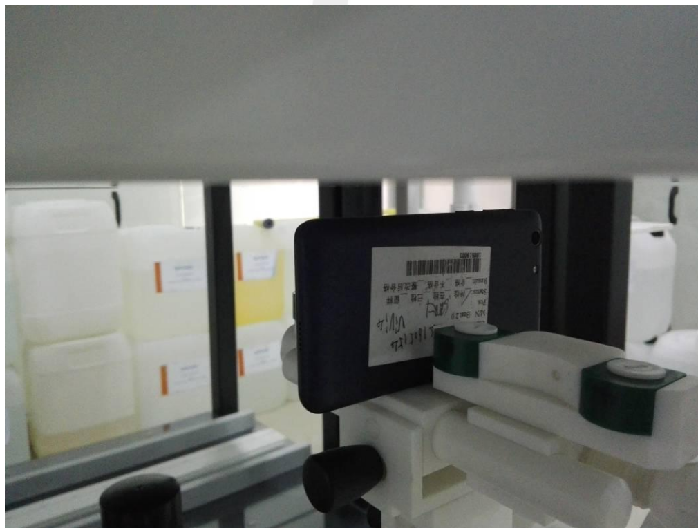
Body right side(separation distance is 10mm)
