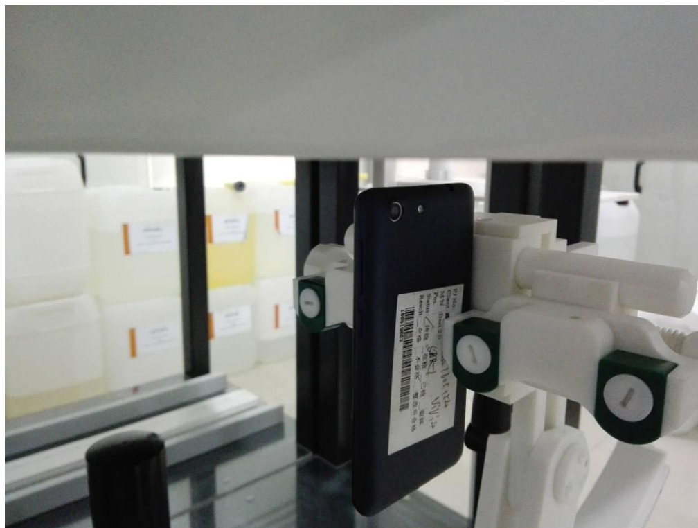
Body top side(separation distance is 10mm)
