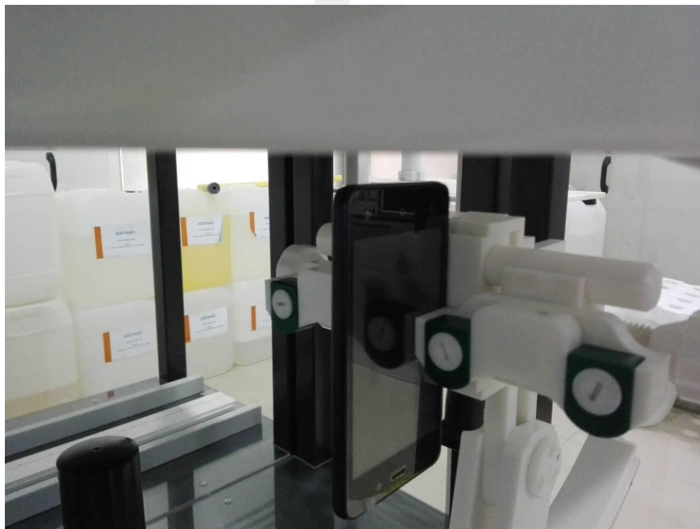
Body Bottom side(separation distance is 10mm)
