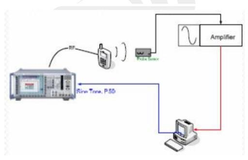
**T-Coil Test Setup**
