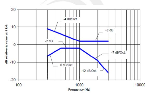
NOTE-The frequency response is between 300 Hz and 3000 Hz.
