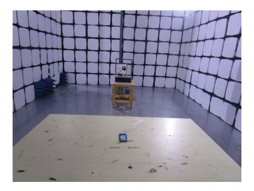
Spurious Radiation Test Setup (30MHz to 1G)
