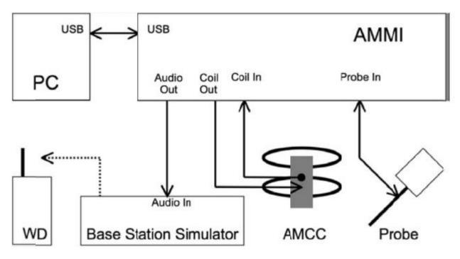
T-Coil setup with HAC Test Arch and AMCC
