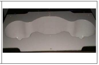
The bottom plate contains three pair of bolts for locking the device holder. The device holder positions are adjusted to the standard measurement positions in the three sections. A white cover is provided to tap the phantom during off-periods to prevent water evaporation and changes in the liquid parameters. On the phantom top, three reference markers are provided to identify the phantom position with respect to the robot.
