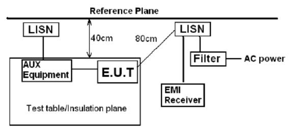
Remark E.U.T: Equipment Under Test LISN: Line Impedence Stabilization Network Test table height=0.8m
