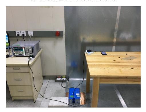
FCC RADIATED EMISSION TEST SETUP
