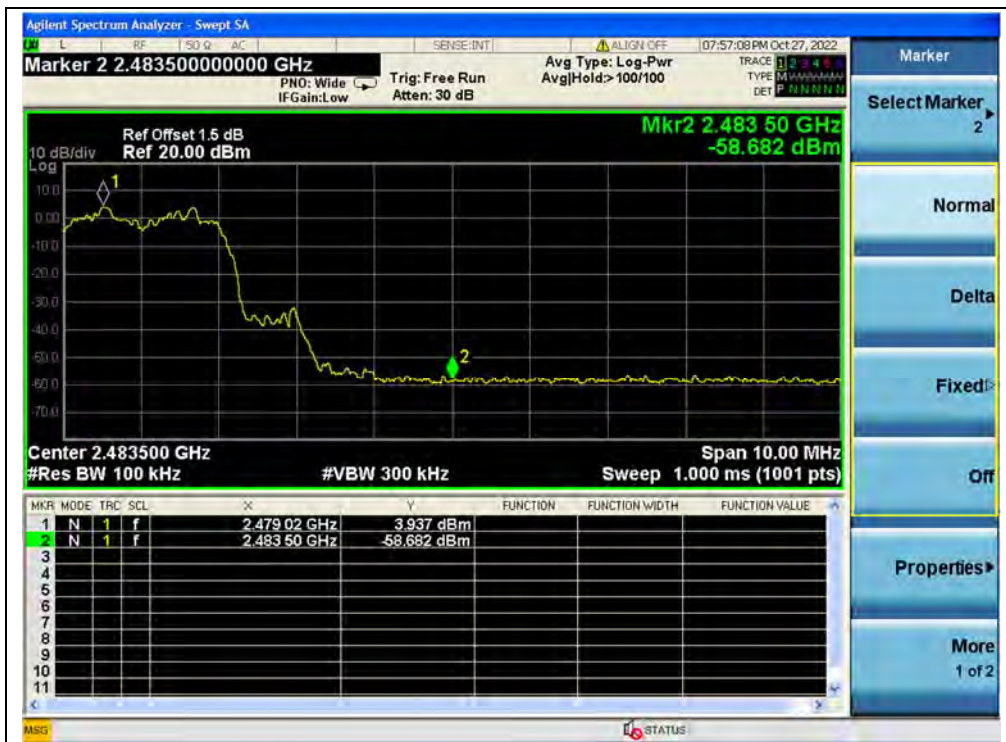
(Band edge with hopping on, Channel 78, 8-DPSK)
