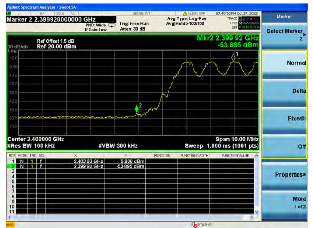
(Band edge with hopping on, Channel 0, GFSK)
