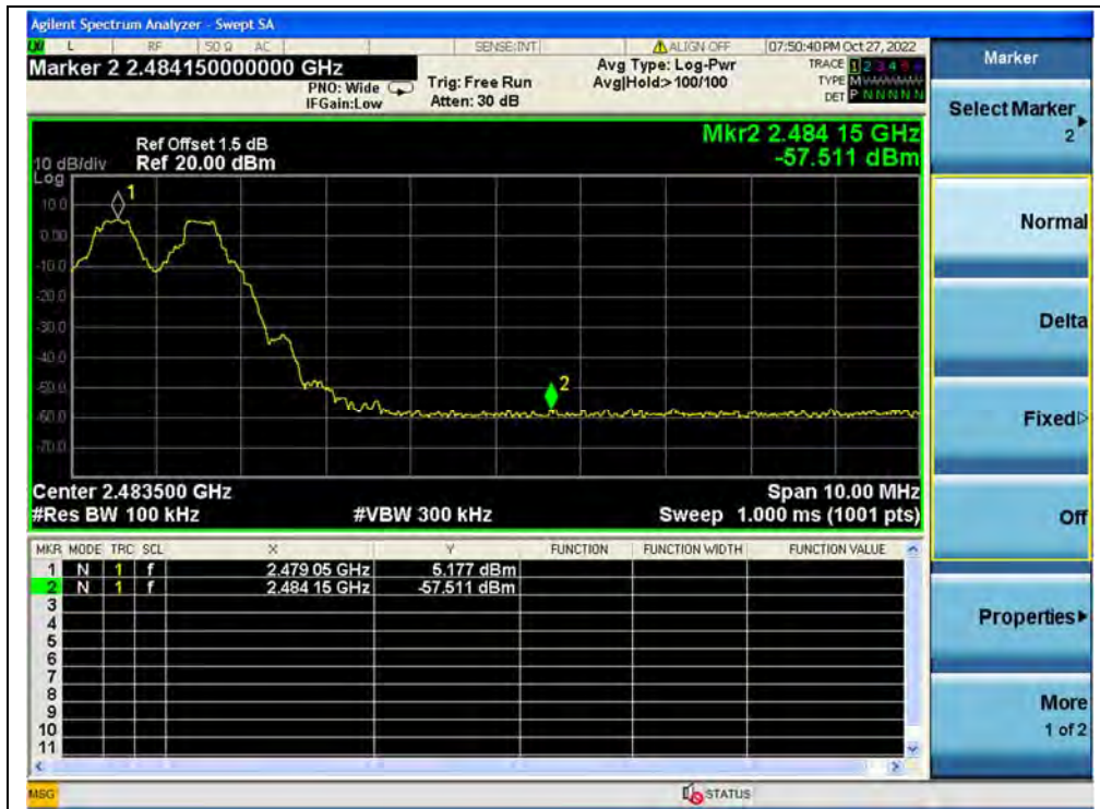
(Band edge with hopping on, Channel 78, GFSK)
