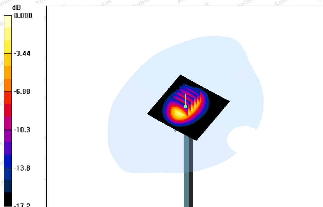
System Performance Check 1900MHz Head 250mW
