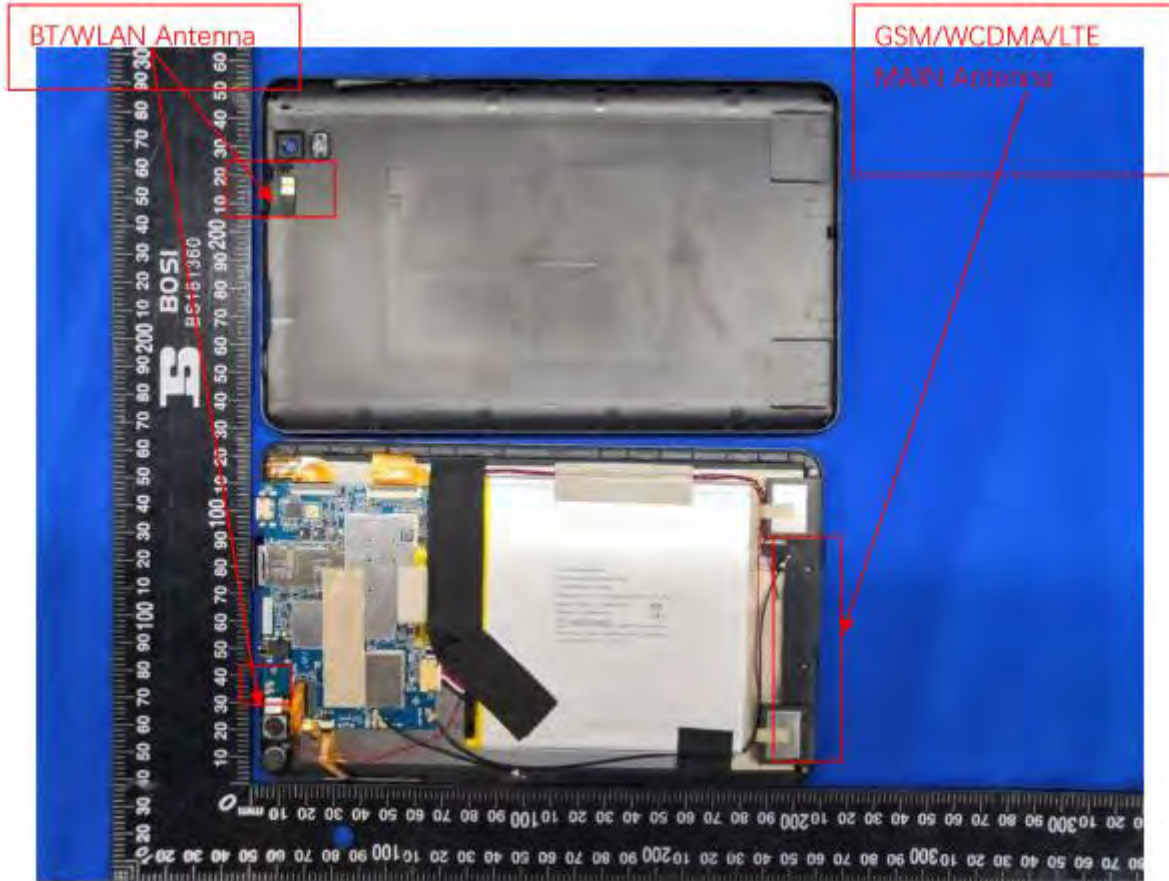
Distance of The Antenna to the EUT surface and edge
