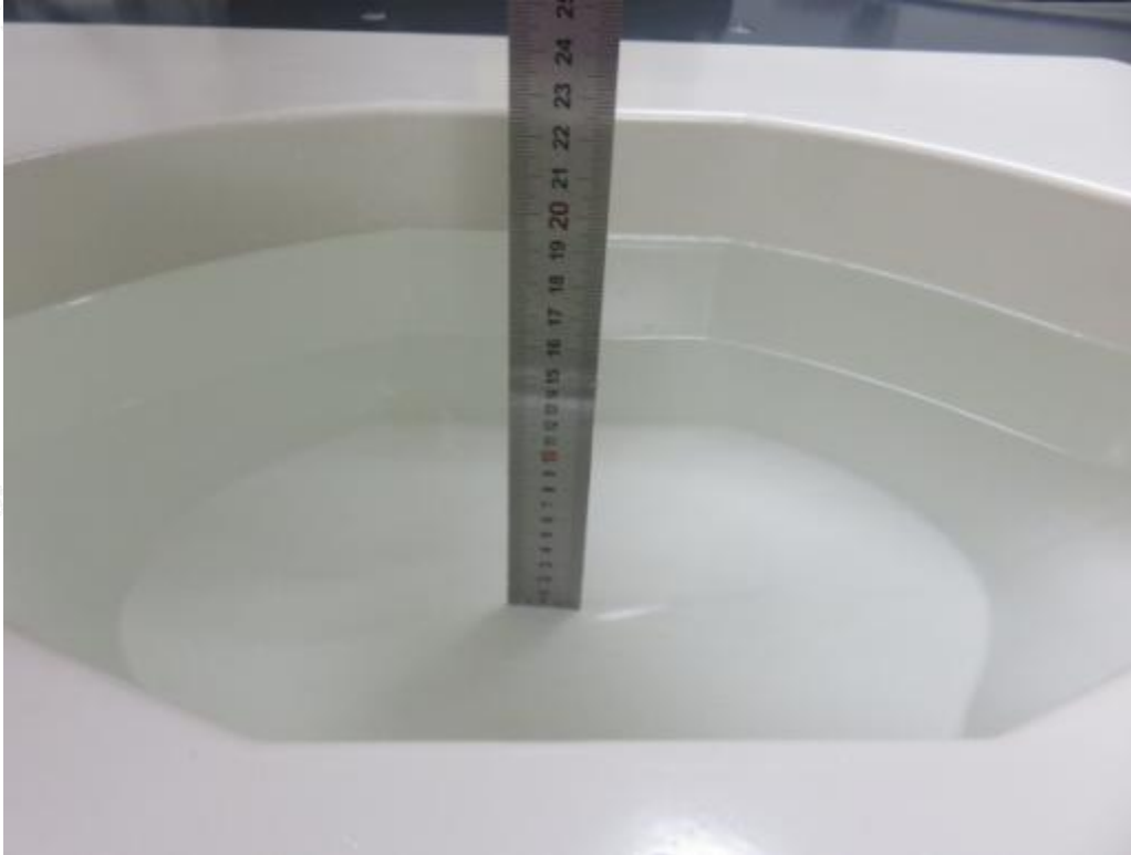
Photograph of the depth in the Body Phantom (1800MHz, 16.1cm depth)
