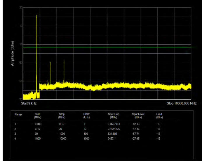
Band26(814-824) 16QAM BW=1.4MHz Channel=26783 RB Size=6 Position=#0
