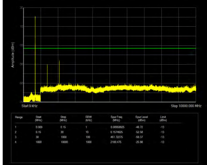
Band12 16QAM BW=1.4MHz Channel=23095 RB Size=6 Position=#0
