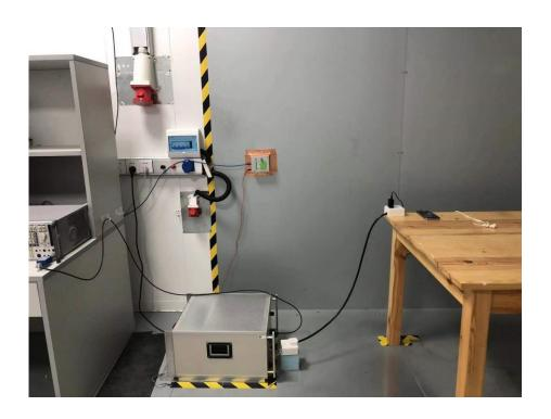
Set-up for Radiated Emission (RE), Below 1GHz
