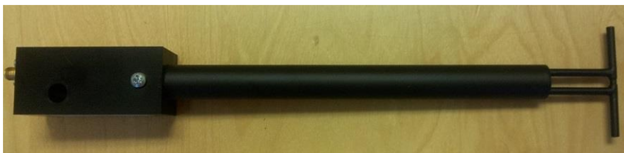
Figure 1 – MVG COMOSAR Validation Dipole
