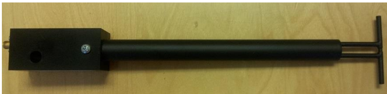
Figure 1 – MVG COMOSAR Validation Dipole
