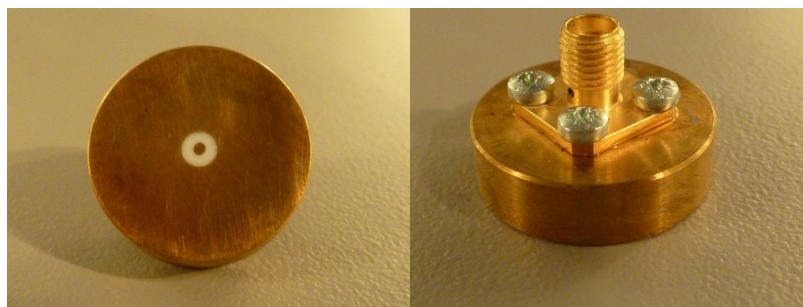
Figure 1 – MVG LIMESAR Dielectric Probe
