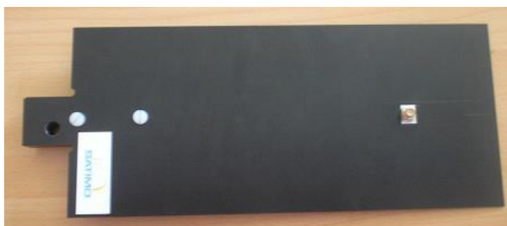
Figure 1 – MVG COMOHAC Validation Dipole
