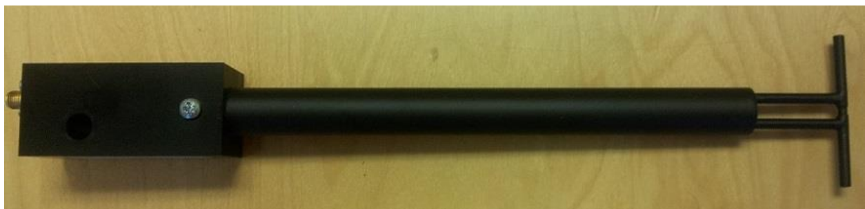
Figure 1 – MVG COMOSAR Validation Dipole
