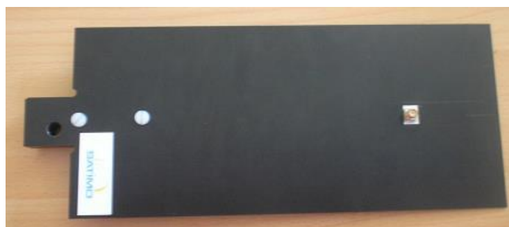
Figure 1 – MVG COMOHAC Validation Dipole
