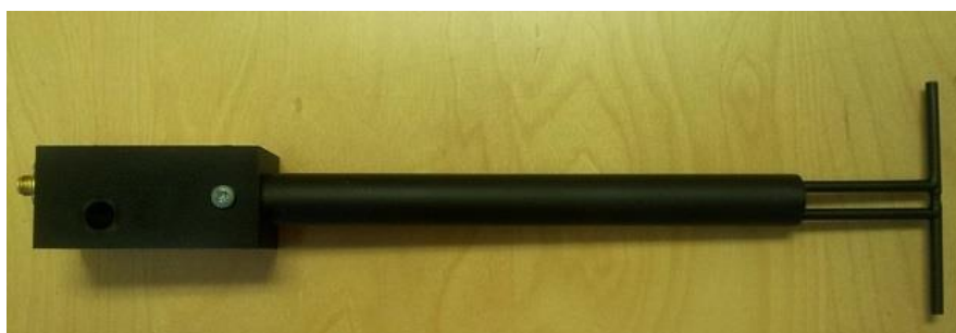
Figure 1 – MVG COMOSAR Validation Dipole
