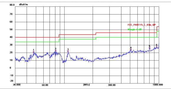
TM1 / Polarization: Vertical / Band: 2.4G / BW: 1 / CH: H
