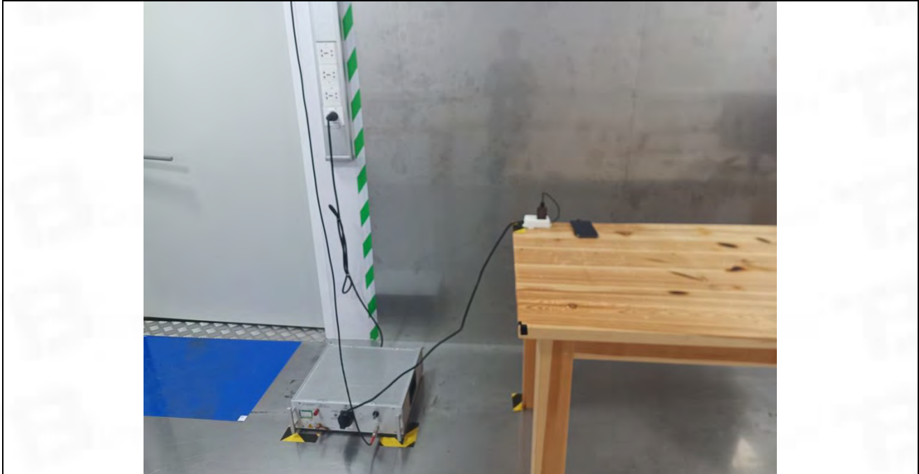
Conducted Emission at AC power line
