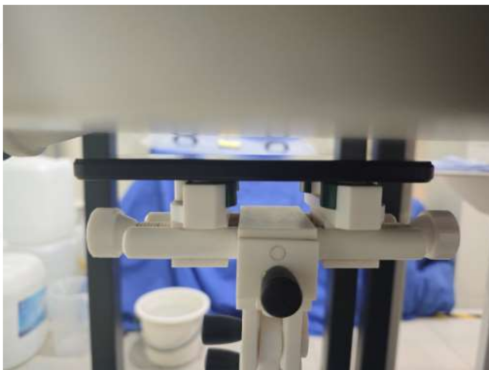
Body Front side(separation distance is 10mm)
