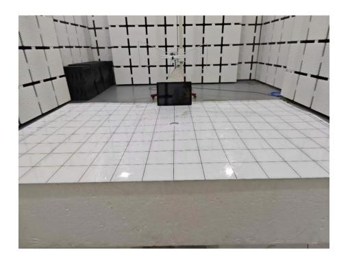
Set-up for Radiated Spurious Emission, Above 1GHz
