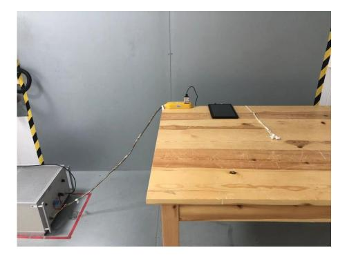
Set-up for Radiated Emission (RE), Below 1GHz
