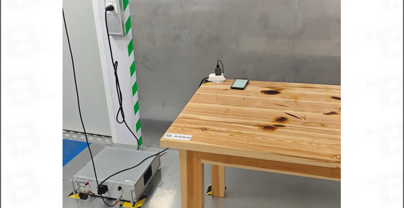
Conducted Emission at AC power line
