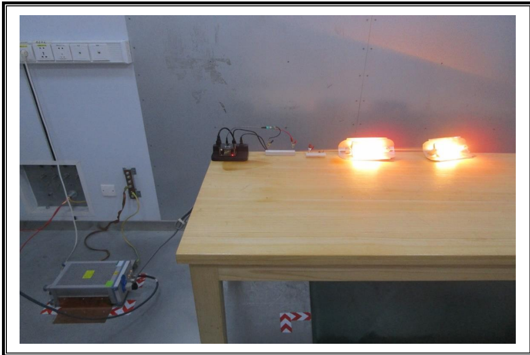
POWERLINE CONDUCTED EMISSIONS MEASUREMENT SETUP
