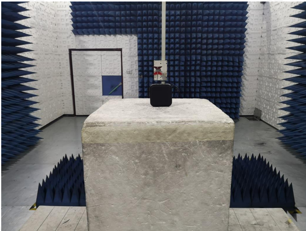
RADIATED EMISSION TEST SETUP ABOVE 1GHZ
