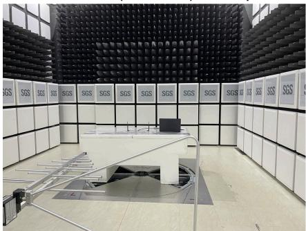
Radiated Emissions (Above 1GHz) Test Setup
