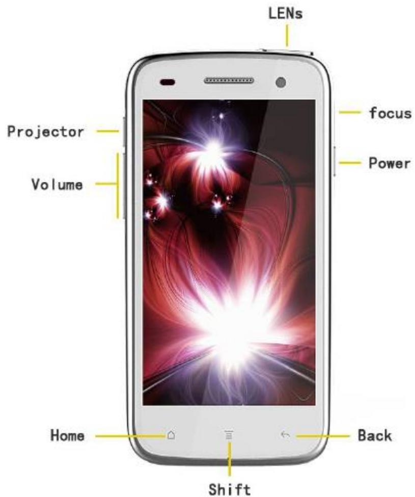
Power, To turn on/off, or screen lock/unlock
