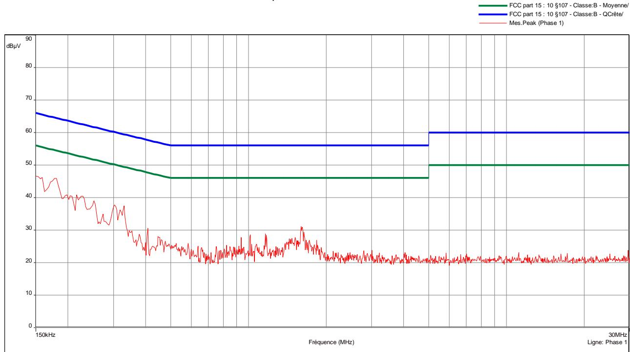
The frequencies which are not 6 dB under the Average limit are then analyzed with Average detector.
