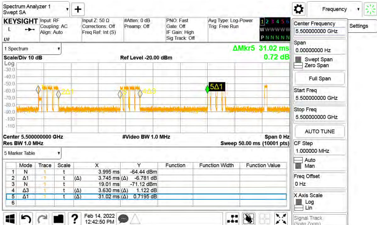
Plot of WLAN Traffic - 802.11ac (20 MHz), 5500 MHz
