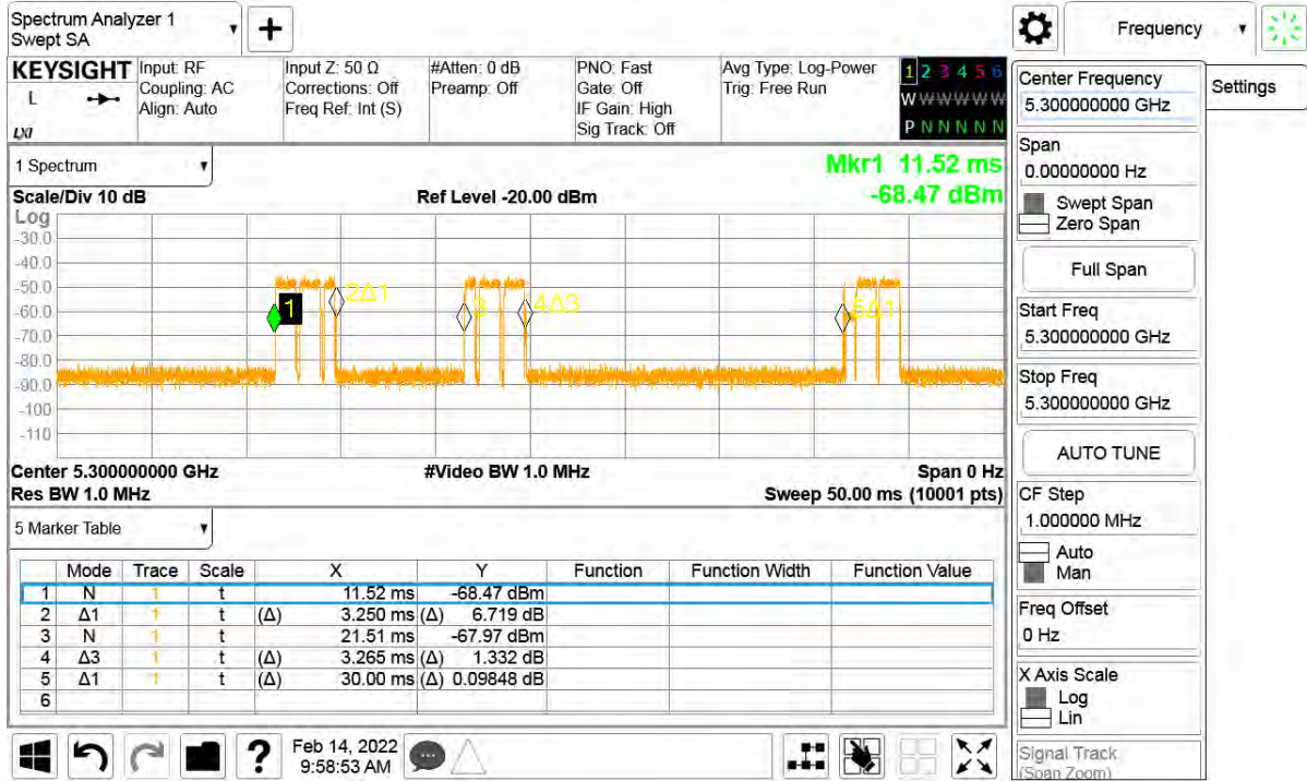
Plot of WLAN Traffic - 802.11ac (20 MHz), 5300 MHz
