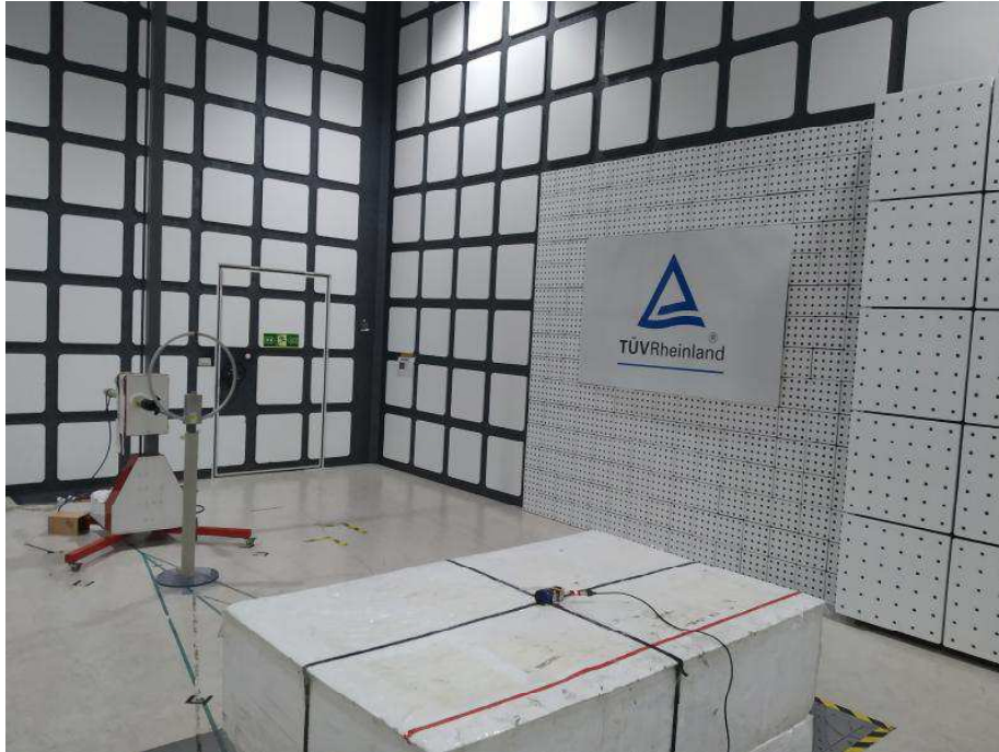
Photograph 5: Set-up for Spurious Emissions (Back View 3)
