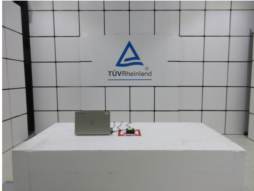
Photograph 1: Set-up for Spurious Emissions (Front View 1)
