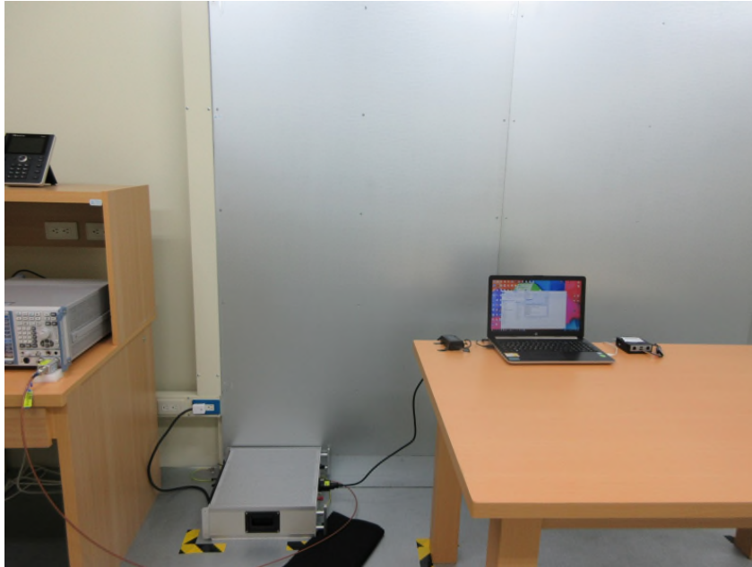
Photograph 7: Set-up for AC Mains (Front View)
