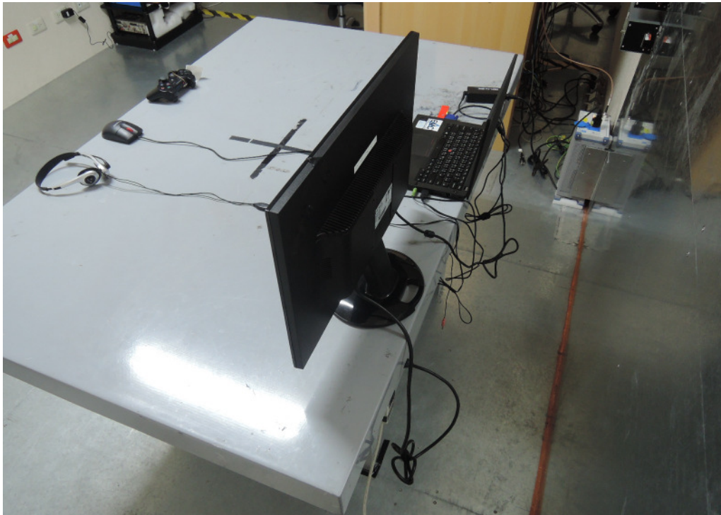
Photograph 5: Set-up for for Mains Conducted testing Back
