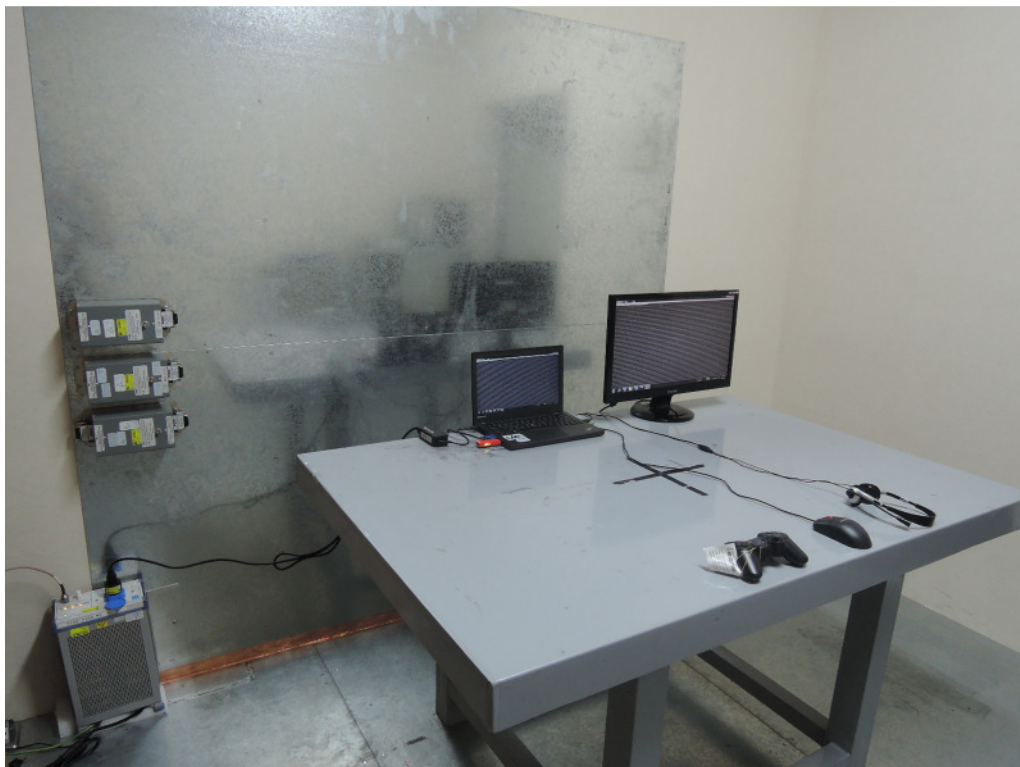
Photograph 6: Set-up for for Mains Conducted testing Front
