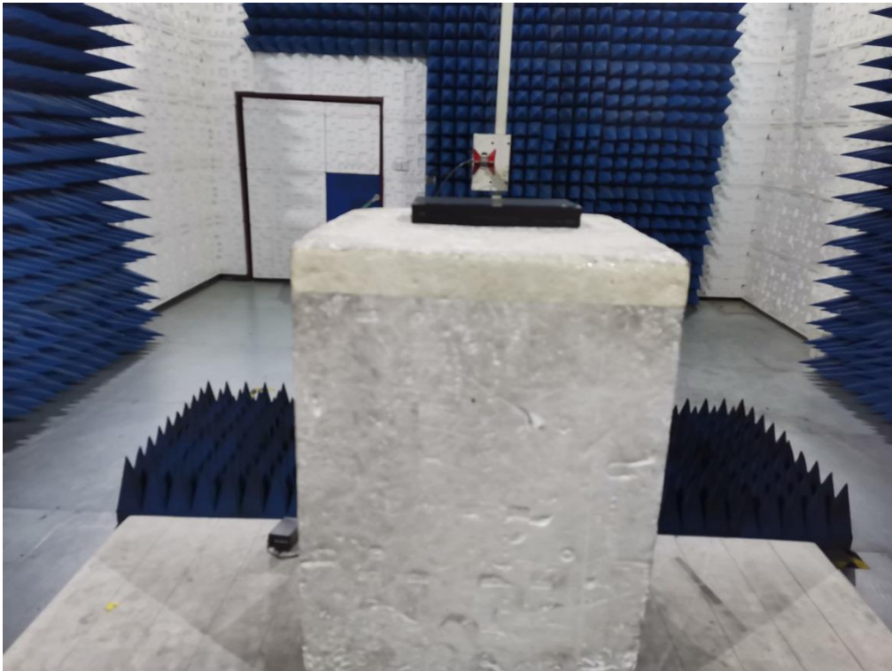
RADIATED EMISSION TEST SETUP ABOVE 1GHZ
