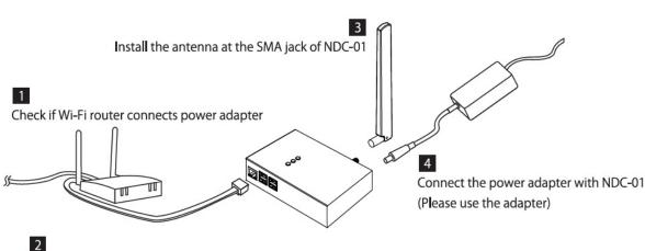
Connect Ethernet cable with the Wi-Fi router, and the other end connects NDC-01
