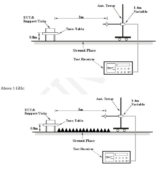
The radiated emission and out of band emission tests were performed in the 3 meters chamber test site, using the setup accordance with the ANSI C63.4-2003. The specification used was the FCC 15.209/15.205 and FCC 15.249 limits.
