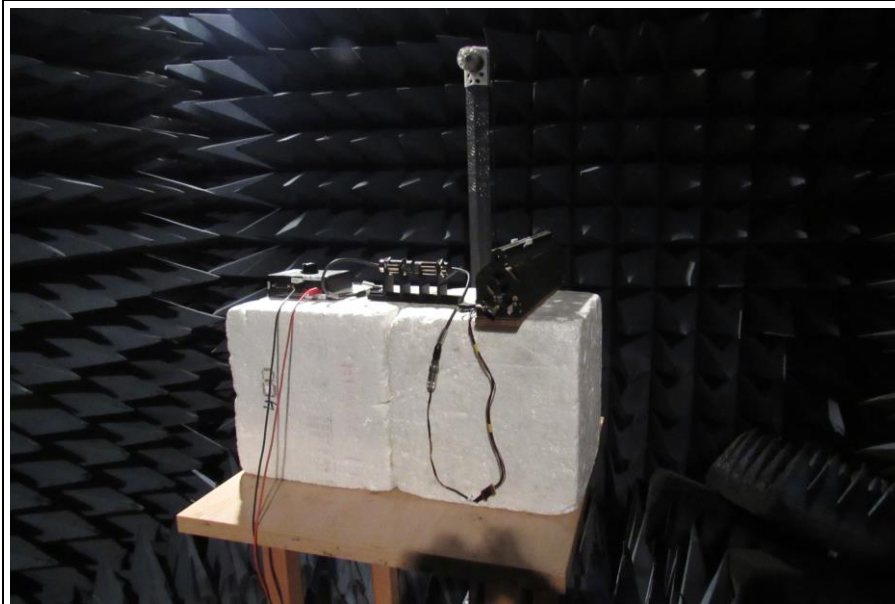
Setup radiated emission below 30 MHz Detail
