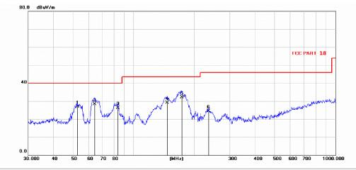
Site LAB Limit: FCC PART 18 Polarization: Horizont
