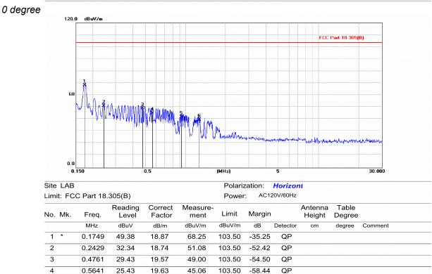
\*Note: 1). Pre-scan all modes and recorded the worst case results in this report. 2). Emission level (dBuV/m) = 20 log Emission level (uV/m).
