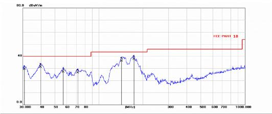
Site LAB Polarization: Vertical Limit: FCC PART 18 AC120V/60Hz Power: Reading Correct Measure-Antenna Table No. Mk. Limit Margin Degree Freq. Height Level Factor ment MHz dBuV dB/m dBuV/m dBuV/m dB Detector degree Comment cm 1 30.8129 16.15 13.11 29.26 40.00 -10.74 QP 2 39.6625 17.00 14.02 31.02 40.00 -8.98 OP 3 56.8914 14.04 13.05 27.09 40.00 -12.91 QP QP 4 71.3300 15.65 10.89 26.54 40.00 -13.46 5 -7.45 QP 142.8870 23.05 13.00 36.05 43.50 6 \* 173.3570 25.04 12.58 37.62 43.50 -5.88 QP
