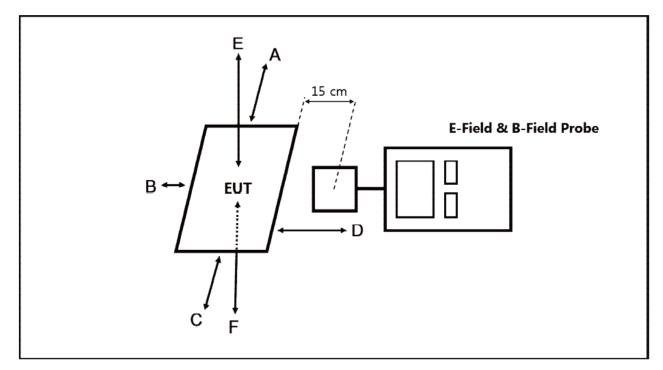
Note: Measurements should be made from all sides and the top of the primary/client pair, with the 10cm measured from the center of the probe(s) to the edge of the device.
