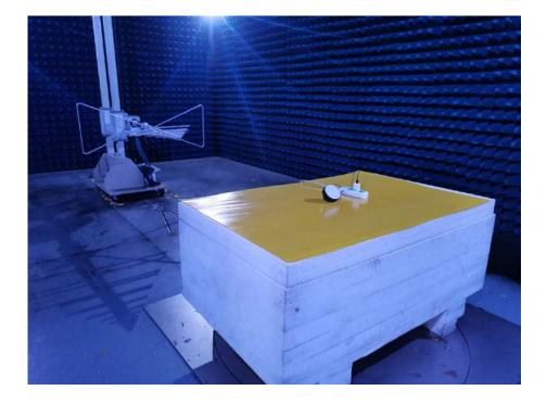
Photo of Radiated Emission Measurement Above 1GHz
