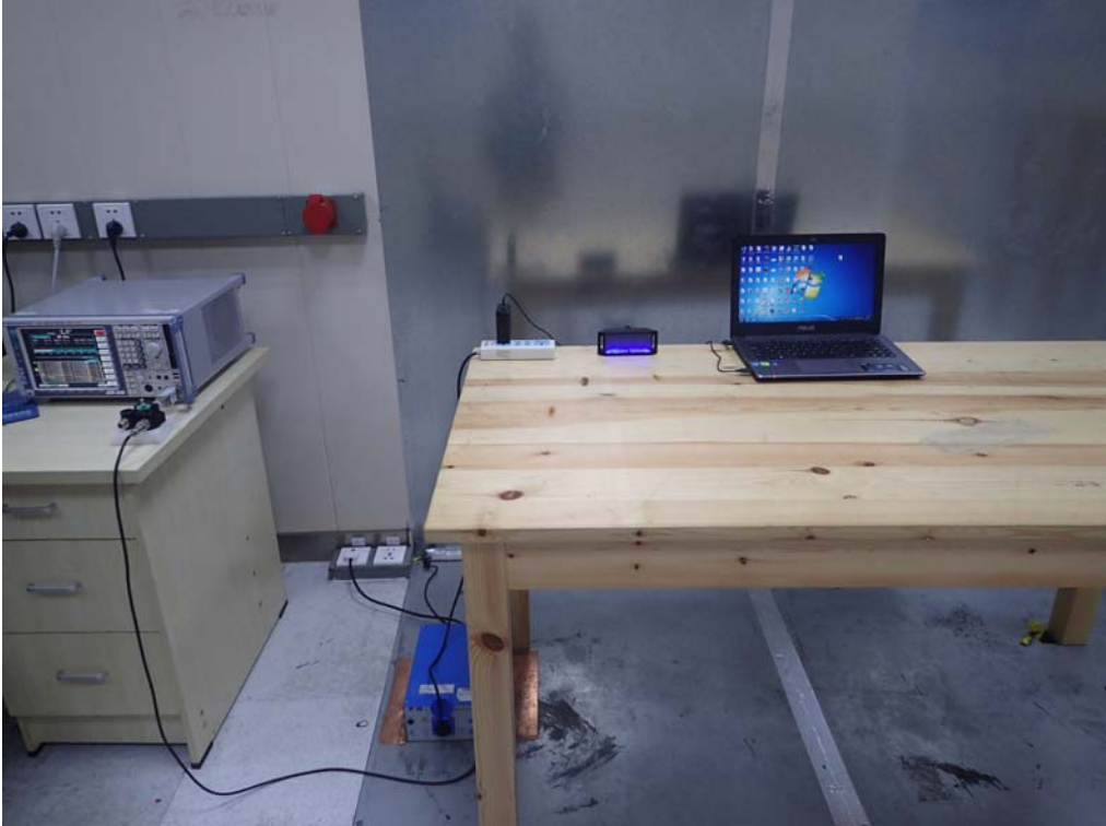
FCC RADIATED EMISSION TEST SETUP
