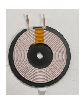
Note: Wrap 8MM (ref) high temperature adhesive paper around coil outlet position
