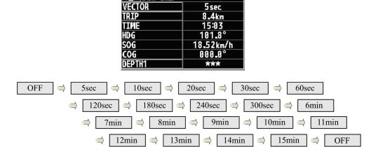
There are shown 2 vectors, one drawn from the bow and the other one from the stern. The vector will be straight when the vessel doesn't turn and curved when the vessel turns.
