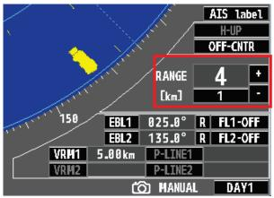
In this case, the distance interval of The Range Rings is 1km.
