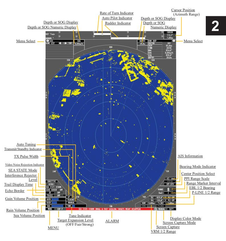
FIG 2.1 DISPLAY & READOUTS
