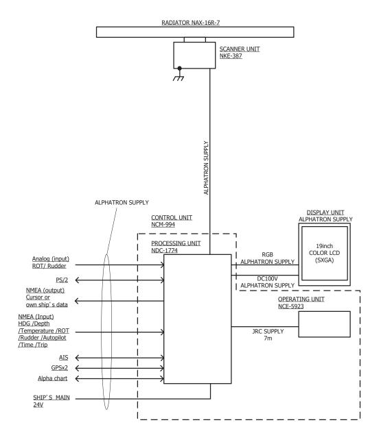
Fig. 1.4 General System Diagram of Radar, Type JMR-611
