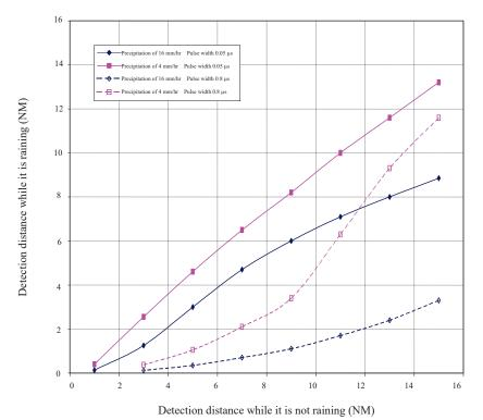
Figure 5.4 Decreased target detection distance due to precipitation
