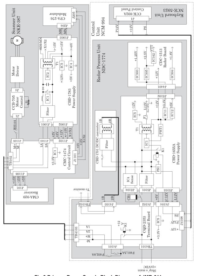
Fig.3 Primary Power Supply Block Diagram of JMR-611
