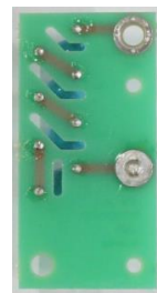
CFR-259 ( Magnetron Filter Circuit ) Parts and Solder Side
