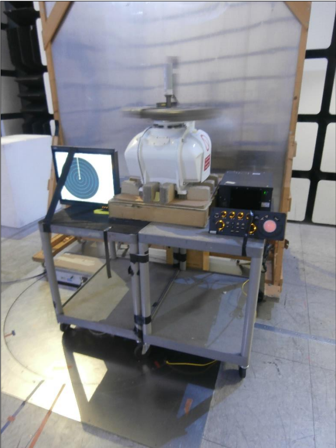
Figure 12 - Test Setup for Conducted Emissions at Mains Terminals
