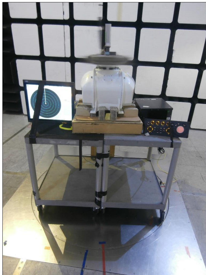
Figure 10 - Test Setup – Antenna Rotating
