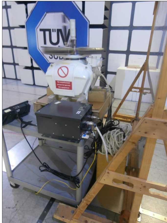
Figure 11 - Test Setup for Conducted Emissions at Mains Terminals
