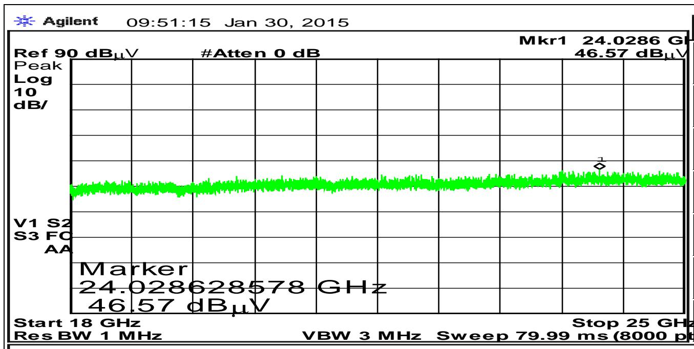
Spec Margin = E-Field Value - Limit, E-Field Value = FIM Value - Amp Gain + Cable Loss + ANT Factor  $\pm$  Uncertainty
