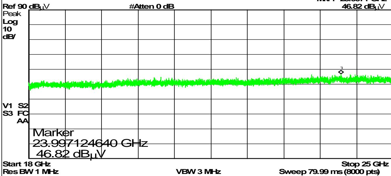
Spec Margin = E-Field Value - Limit, E-Field Value = FIM Value - Amp Gain + Cable Loss + ANT Factor  $\pm$  Uncertainty
