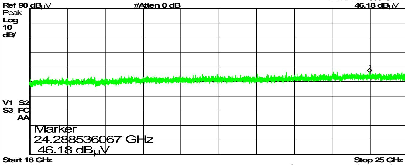
Spec Margin = E-Field Value - Limit, E-Field Value = FIM Value - Amp Gain + Cable Loss + ANT Factor  $\pm$  Uncertainty
