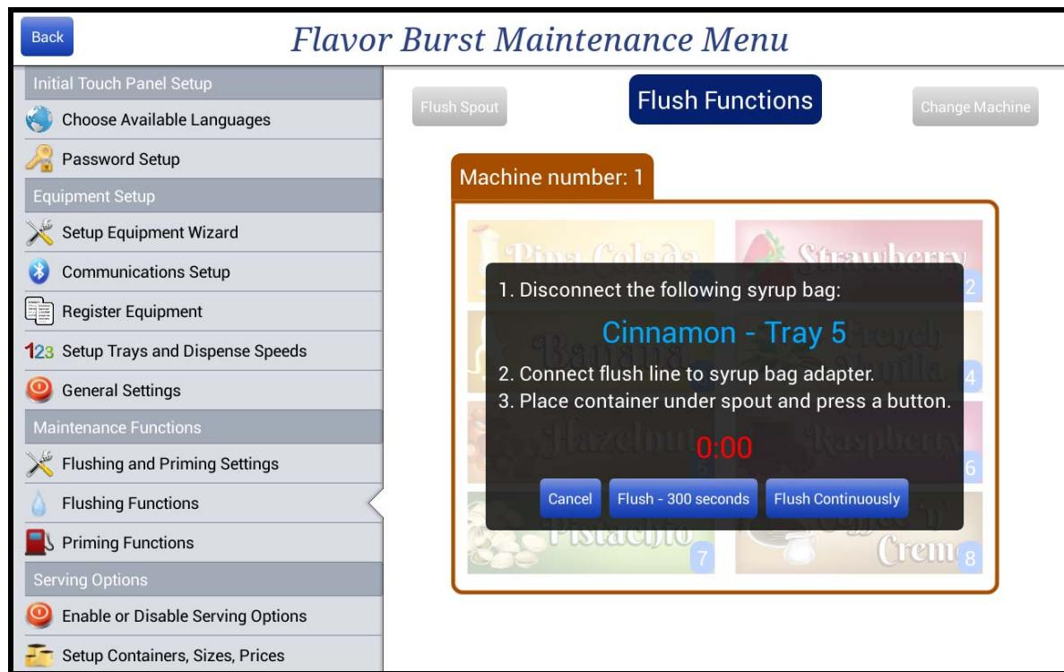
This screen allows the operator to flush a line with sanitizer or flush the head with sanitizer or water. If there is more than one cabinet of syrups installed on this touch panel, a "Change Machine" button will be displayed at the upper right-hand corner of the screen. This will give the operator an opportunity to perform the same functions on the second machine.
