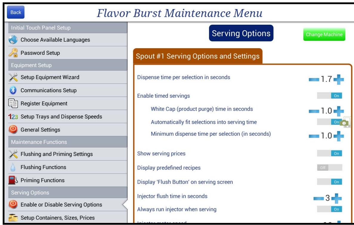
The operator can set serving-specific options on this screen. If there is more than one cabinet of syrups installed on this touch panel dispensing to two spouts, a "Change Machine" button will be displayed at the upper right-hand corner of the screen. This will give the operator an opportunity to perform the same functions on the second machine. Certain machine configurations will prevent some of the functions listed here from being displayed.
