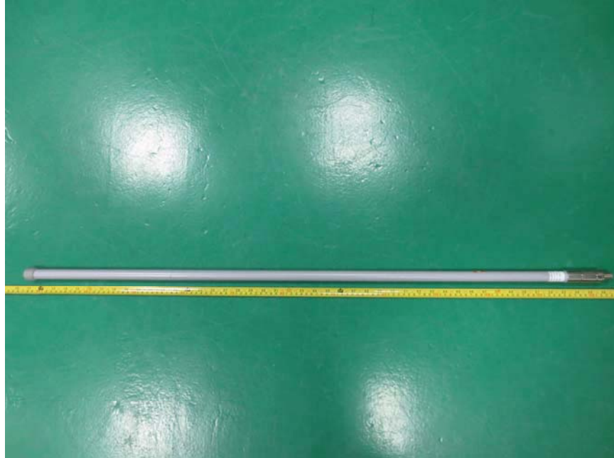
12dBi omni-directional antenna
